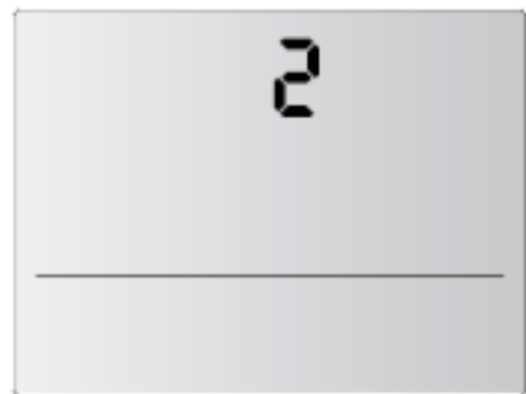
2 units connected to the control (last number shown during initialization)
